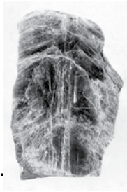
A. Cleavage in one direction. Example: Muscovite.
