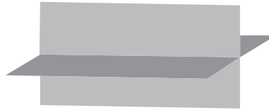
B. Cleavage in two directions at right angles. Example: Feldspar.
