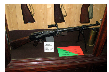
The Belgian-made FN Mle D variant with quick-change barrel.
