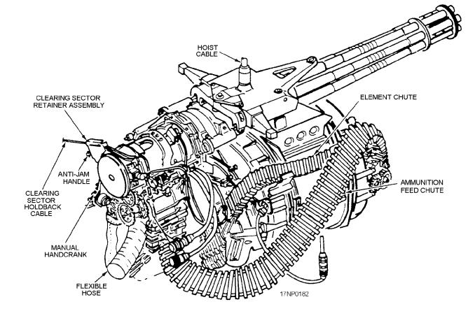
Figure 6-14.—F/A-18 M61A1 gun installation.
