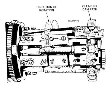
Figure 6-11.—Breech-bolt assembly in clearing cycle.
