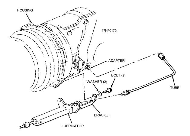
Figure 6-7.—Lubricator assembly installation (F-14).
