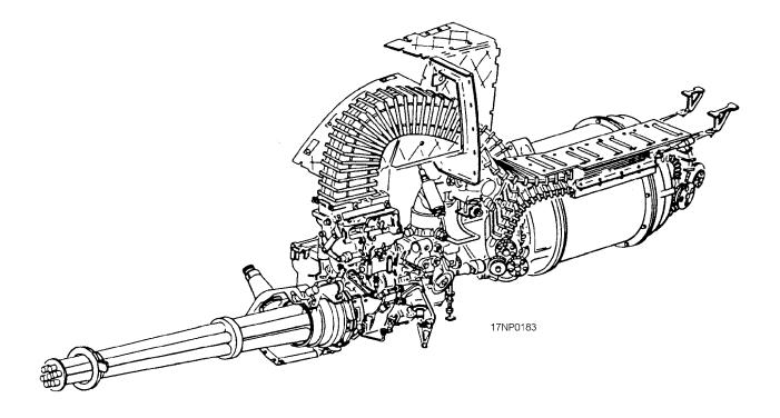
Figure 6-15.—F-14 M61A1 gun installation.
