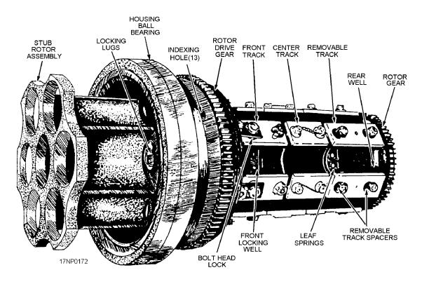
Figure 6-4.—Rotor assembly.
