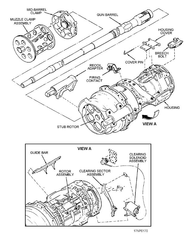
Figure 6-2.—Gun components (exploded view).
