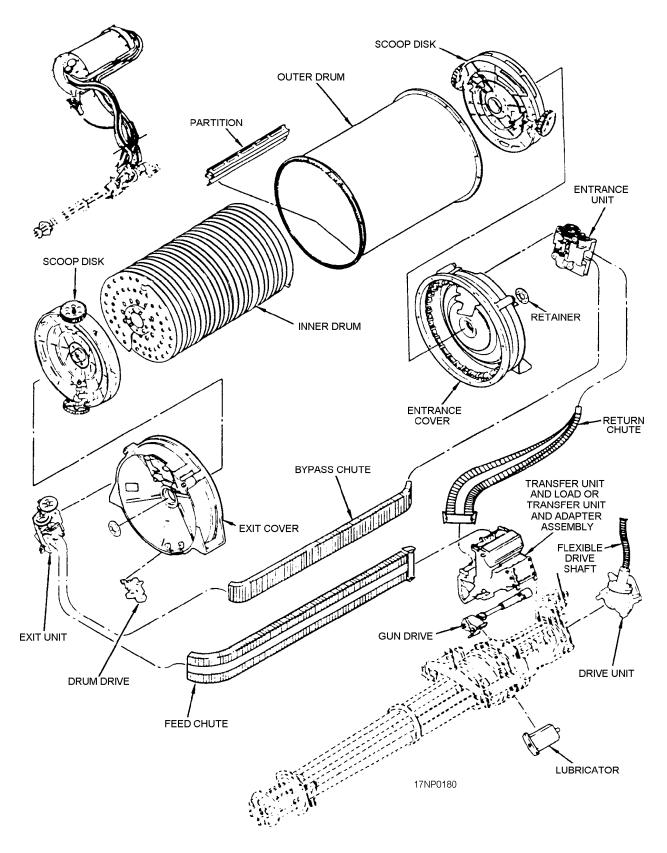
Figure 6-12.—Ammunition handling components (exploded view).
