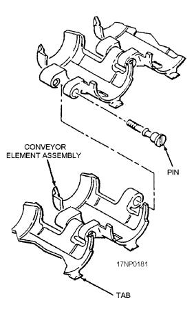
Figure 6-13.—Typical conveyor element assembly.
