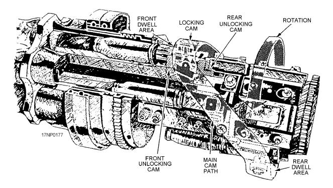
Figure 6-9.—Breech-bolt assembly in firing cycle.
