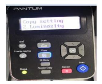
Step6: Select "No.1-Custom/ manual" and adjust to full dark by press direction pad "▲" will be done.
