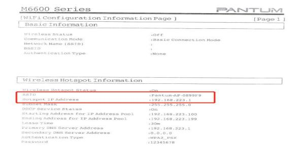
**Step2:** Make sure that the printer "Wi-Fi" button is turn on, then connect the IOS mobile device with wireless network of the printer SSID, the default password is 12345678
