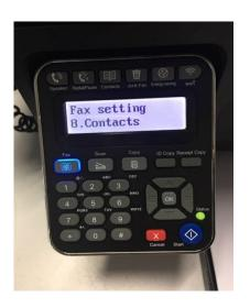
**Step4:** Enter the fax number one by one by pressing the number on the "NO.4 New and edit"
