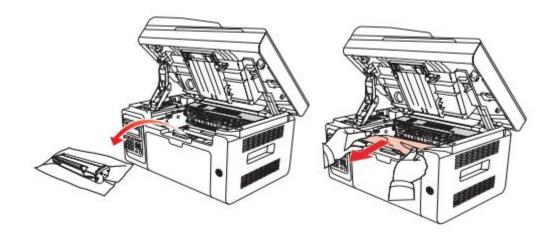
**Step3:** After removing the jammed paper, insert the laser toner cartridge into the printer along the guides until you hear a "click" assuring you that the cartridge is fully inserted.
