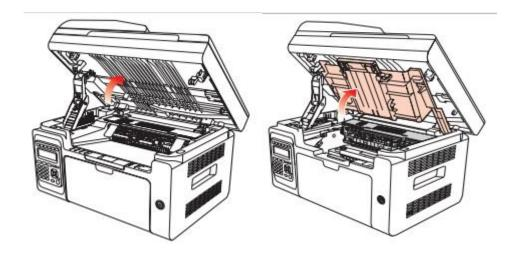
**Step2:** Remove the laser toner cartridge along the guides. Gently draw the jammed paper out along the paper output direction.
