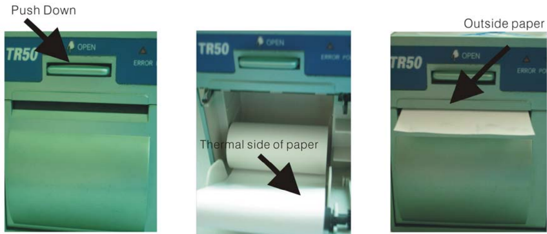
Fig. 3-6-1 Install Recording Paper
