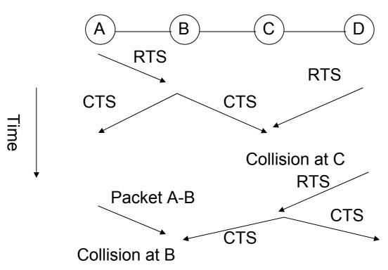
C hears a collision (for CTS) & hence transmits CTS (to D) which collides with packet at node B
