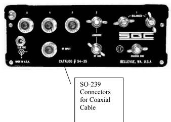
Three SO-239 connectors are provided for antennas fed with Coaxial cable. SGC recommends that one connector be reserved for a dummy load if possible for testing purposes. From the front panel, these three connections correspond to switches 3, 4, and 5.
