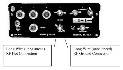
The long wire connection starts from two lugs on the back panel labeled 'Longwire.' They correspond to antenna selection switch 2 on the front panel. An RF ground connects to the lug labeled RF GND. When using a single wire 'counterpoise, it should be 5-10% longer than the random length long wire.
