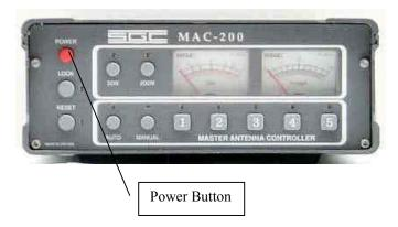
Momentarily press the Red Power button on the front panel to activate the MAC-200. You should see the LEDs behind the meter displays light up.
