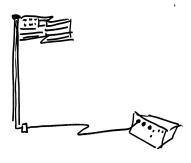
Home made vertical antennas are commonly made in one of two ways. A very common type of construction builds the radial system at the base of the antenna. Flag pole antennas are normally built in this way. Coax line can be run from the MAC-200 to the base of the antenna. The center lead of the coax will feed the radiating
