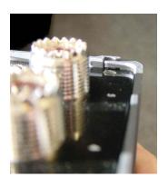
3. Holding the MAC-200 with the back panel UP, push the washer into the slot engaging the cover slot and drive the screw into the hole until tight.
