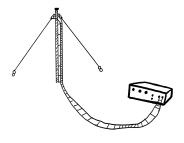
The inverted-V antenna can be fed with ladder line run from the balanced line connection on the MAC-200, but it is also commonly fed from coaxial cable with the center conductor to one side and the shield to the other.
