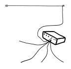
Unbalanced antennas need an RF Ground or counterpoise to create electrical balance and depend on the quality of the ground for a high quality radiated signal. Without a good quality ground, unbalanced antennas will cause interference, lead to RF in the radio room, and be of very low efficiency due to high losses in the ground. Typical
