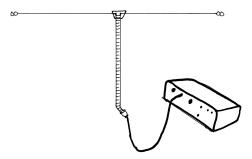
Some antennas, such as the G5RV, use a section of ladder line as a matching device. These transform the impedance of feed point to something near 50 ohms. Usually, the ladder line terminates in a 1:1 balun. The Coaxial line from the transceiver connects to the balun. The MAC-200 can feed this connection directly from one of the coax ports or you can remove the balun run the ladder line directly to the MAC-200 balanced feed line port.
