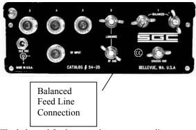
The balanced feed connections corresponding to antenna switch 1, will accept any form of balanced feed line for an external antenna.
