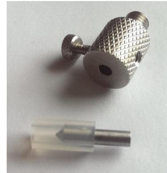
Figure 3. Adaptor (top) and indenter (bottom)
