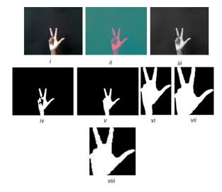
FIGURE II: IMAGE PROCESSING STEPS - (i) Original RGB Sign Image (ii) YCbCr Image (iii) Isolated Channel Representation (iv) Binarized (v) Filled (vi) Bounding Box Around Hand (vii) Wrist Segmented (viii) Resized to 70x70
