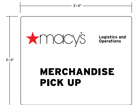
ALUMINUM BLADE SIGN PAINTED WHITE WITH VINYL GRAPHICS APPLIED TO FIRST SURFACE
