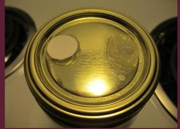
A finished lid for use with spore water or liquid culture, with the tyvek filter on the left
