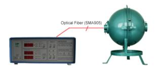
The system can determine spectral power distribution, chromaticity coordinates, correlated color temperature, color rending index(Ra), color difference, wavelength, spectral half width, dominant wavelength, color purity, luminous flux, test for photometery, colorimetry & electricity of LED characteristics.
