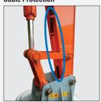
The magnet cable is arranged in the center of the arm top plate for protection against damage by metal debris.
