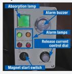
The cab control panel is provided with an array of controls for safe operation.
