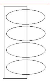
To the left is a picture of the model well use to calculate the magnetic field inside a solenoid. Our model has infinitely many rings not just 4. The current going through the loop is j \* the current going through each loop. The distance between each loop is 1/n = I/N so the perimeter of the loop for Amperes Law is 2R + j/n. Therefore using amperes law the magnetic field in the loop is:
