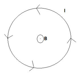
We have a current, I, going counter-clockwise around in a closed loop. From the right hand rule we can see that in the center of the loop the magnetic field points out of the page. Using the Biot-Savart law
