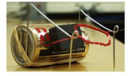
Figure 4: The Completed Electric Motor
