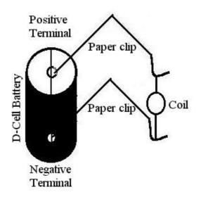
Figure 3: Electric Motor Diagram
