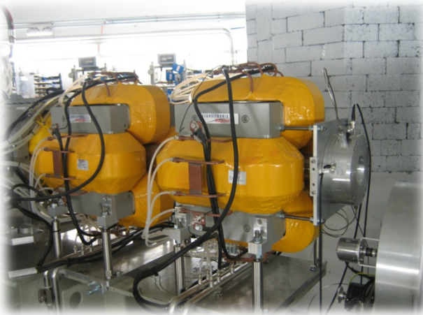
Bending and focusing magnets in particle accelerators (LHC 8.4T!)
