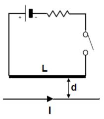
A thin horizontal rod has a length L = 1 m and mass m = 50 g is connected to a circuit. The circuit contains a battery V = 12 V, a resistor R =  $0.06 \Omega$ , a switch, and connecting wires. The rod is supported in horizontal position by two light connecting wires.
