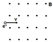
20. An electron with a mass m and charge e enters at a constant speed v a uniform magnetic field B. What is the radius of the curvature of the electron in the field?
