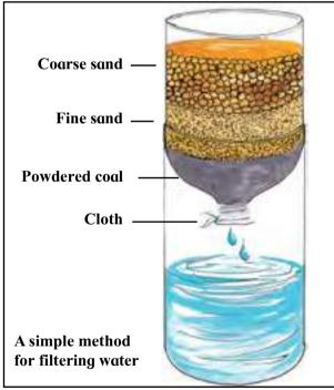
Place the bottle on its lower cut off portion as shown in the figure. Now, pour some muddy water containing some rubbish, slowly into this bottle.
