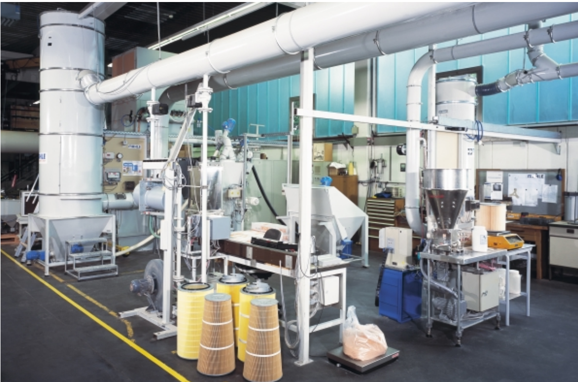
Filter test stand in the MAHLE Industrial Filter Pilot Plant with continuous cleaning and residual dust monitoring.
