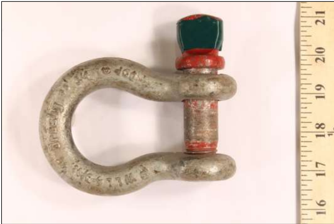
Photo 3 – MATCO photo of Crosby \frac{3}{4} -inch screw pin shackle. Rated working load limit of 4- \frac{3}{4} tons.
