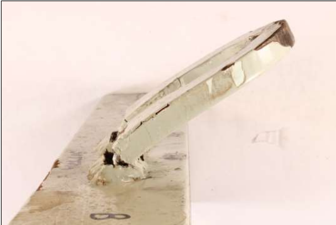
Photo 7 – MATCO photo of deformed shape and fractures after the intact lug was tested at TUV Rheinland. The arrow points in the direction of the top of the door
