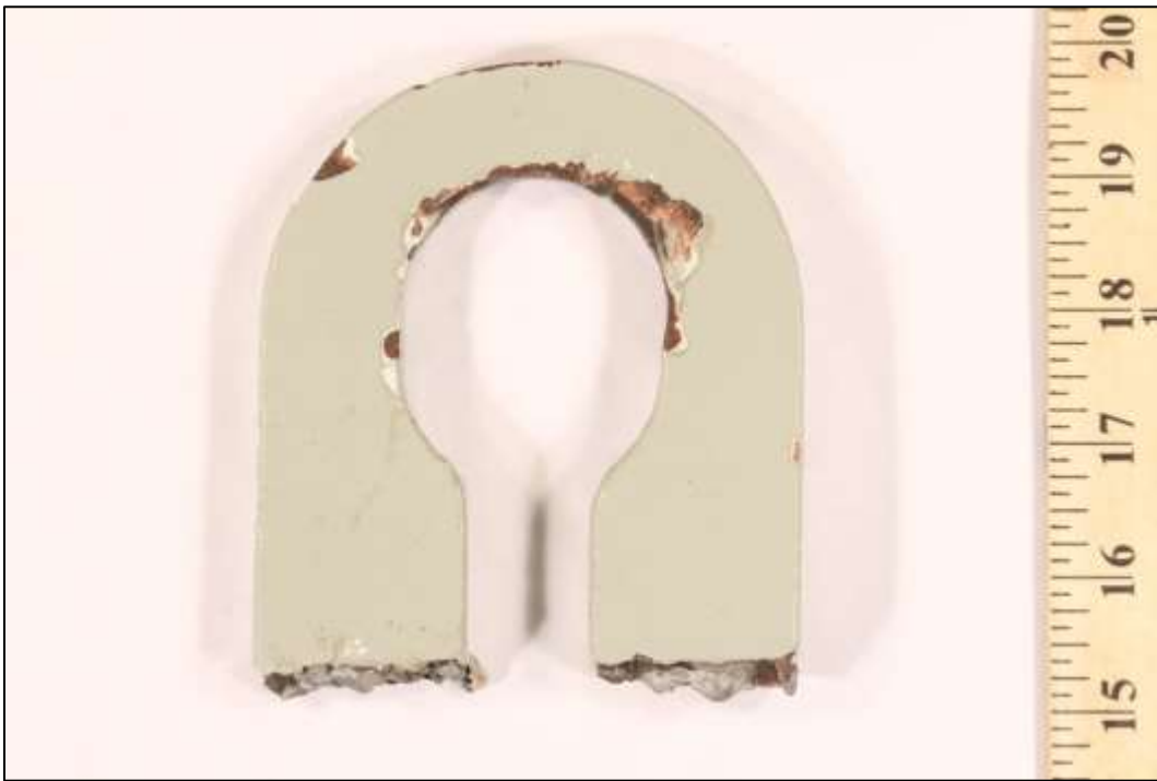
Photo 2 – MATCO photo of the bottom face of the failed lifting lug.
