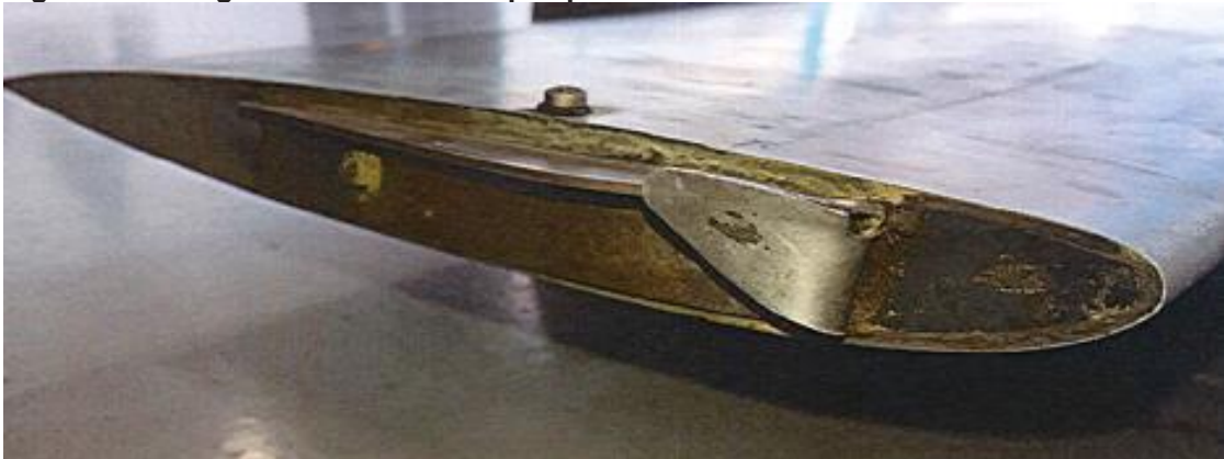
Figure 4: Damage to VH-PHU rotor tip caps
