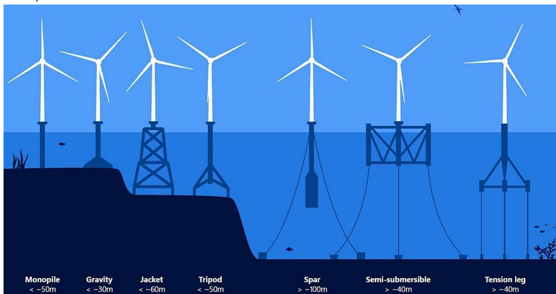
Figure 3-1. Fixed-bottom and floating offshore wind foundations illustration, DHI/Wind Resources and Transmission Lines, NREL
