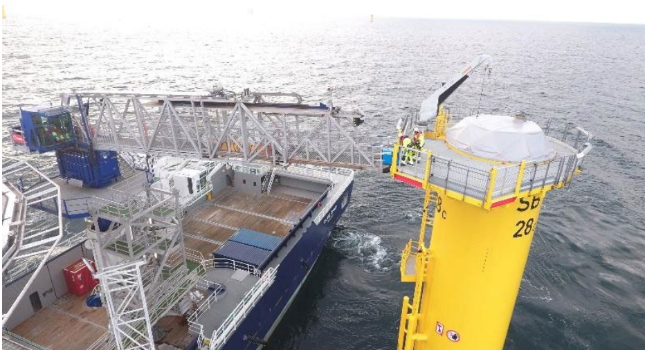
Figure 5-9. Walk to work motion-compensated platform
