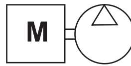
Reciprocating engine and compressor
