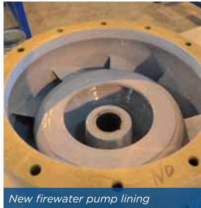
Impeller protected with Belzona lining
