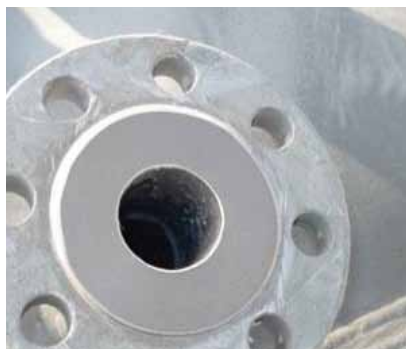
Cold forming isolates flange faces from corrosive media
