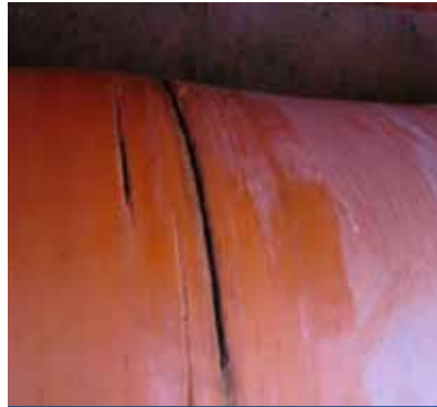
Hose damaged in transport
