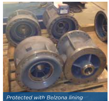
Impeller protected with Belzona lining
