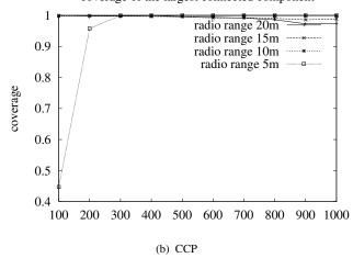
FIGURE 16 Coverage of the largest connected component versus the number of sensor nodes deployed with respect to different radio ranges under OGDC and CCP (the sensing range is fixed at 10m).
