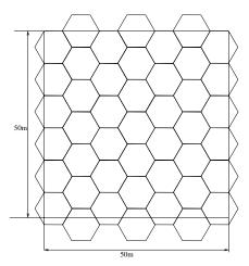
FIGURE 9 45 hexagons are required to cover a  $50 \times 50 \text{ m}^2$  area.
