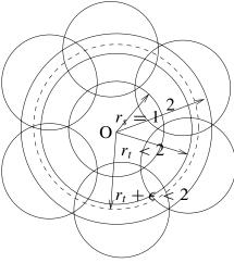
FIGURE 1 A scenario that demonstrates  $r_t \ge 2r_s$  is a necessary condition that complete coverage ensures connectivity.
