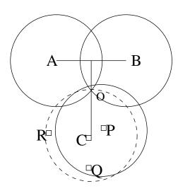
FIGURE 4 Although C is the optimal place to cover the crossing O of A, B, there is no sensor node there. The node closest to C, P, is selected to cover the crossing O.
