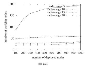
Number of working nodes versus number of sensor nodes deployed with respect to different radio ranges under OGDC and CCP (the sensing range is fixed at 10m).
