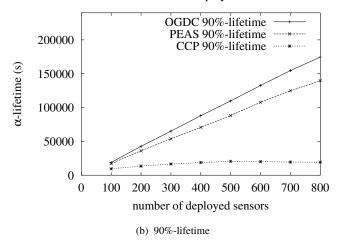
FIGURE 13 Comparison of  $\alpha$ -lifetime versus number of sensor nodes under OGDC, PEAS (with probing
