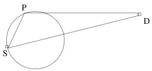
FIGURE 2 A scenario that demonstrates  $r_t \ge 2r_s$  is the sufficient condition that complete coverage implies connectivity.
