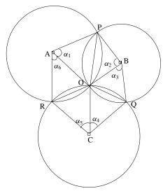
FIGURE 5 Minimizing the overlap while covering the crossing point O when each node has different sensing range.
