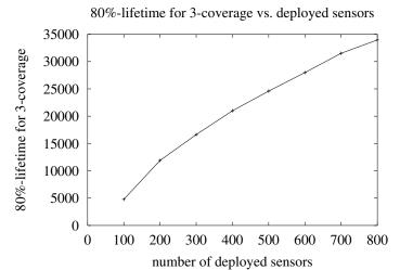
FIGURE 14 80%-lifetime with 3-coverage versus number of sensor nodes under OGDC.
