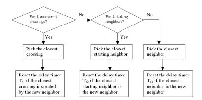
FIGURE 6 The procedure taken when a node receives a power-on message
