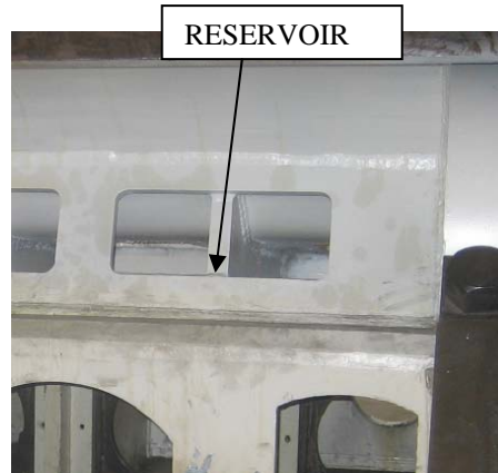
Fig. 2-2 Secondary lubricating system.
