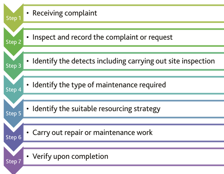
Figure 7.1: Standard Operating Procedure (SOP) for Buildings
