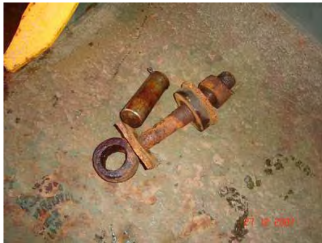
Bent securing device
