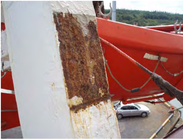
Corrosion of lifeboat davit
