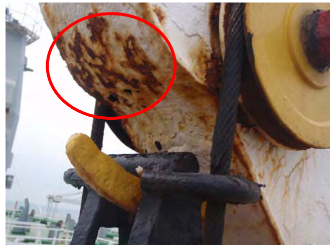
Corrosion of lifeboat davit
