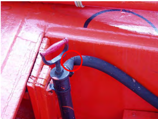
Cracked hose of bilge pump
