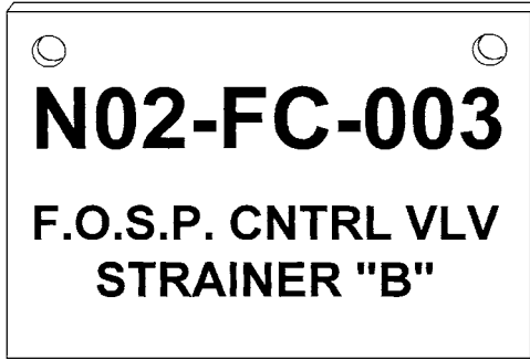
Figure K.4 Example of 2 3 3-inch equipment tag for North Station Unit no. 2 Fuel Oil Service Pump Control Valve Strainer B.
