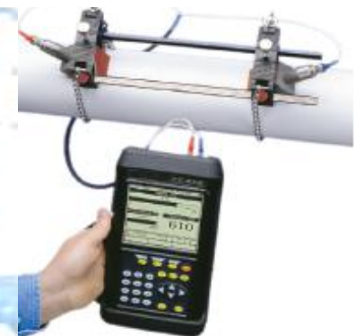
Transit-time flow measurement technique
