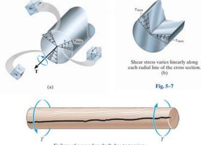
Failure of a wooden shaft due to torsion.
