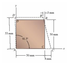
The plate distorts into the dashed position shown. Determine
