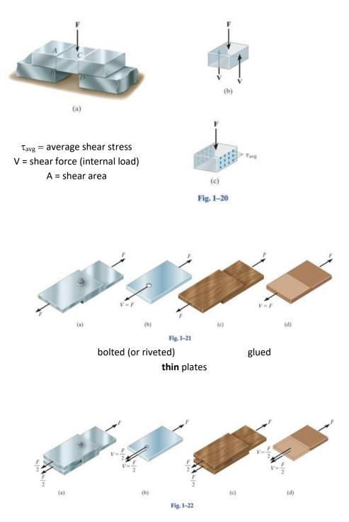
As the plates are **thin**, the bending moment due to F can be neglected. For thick plates, F will have a bending effect in addition to shearing.
