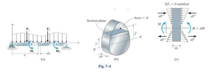
Concentrate on a section that is y' distance away from the neutral axis.
