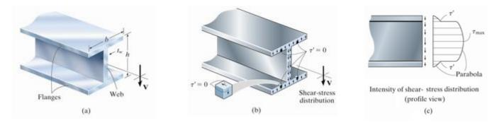
As the thickness changes instantly A **jump** occurs in shear stress distribution Example 1: For the cross section shown,
