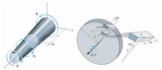
Constant torque and cross section
