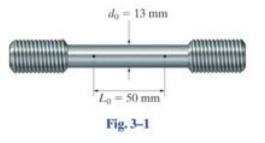
Used primarily to determine the relationship between the average normal stress and the average normal strain
