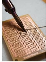
**1e.** Install the 0.01µF capacitor so one leg connects to pin 2 of the chip and one leg is in a "proto row." Flip it over and solder it
