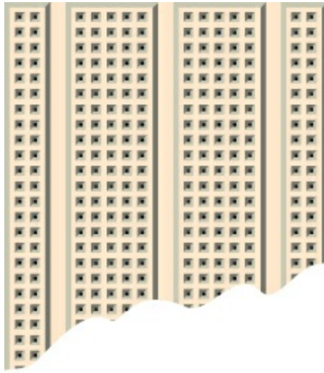
Figure 2-72. A typical breadboard. You can plug components into the holes to test a circuit very quickly.
