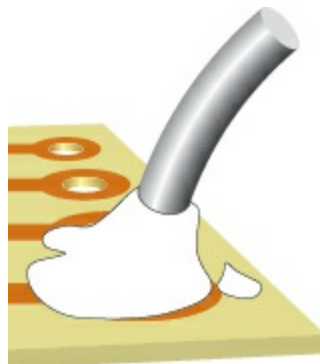
Figure 3-101. If too much solder is used, it makes a mess and can create an unwanted connection with another
