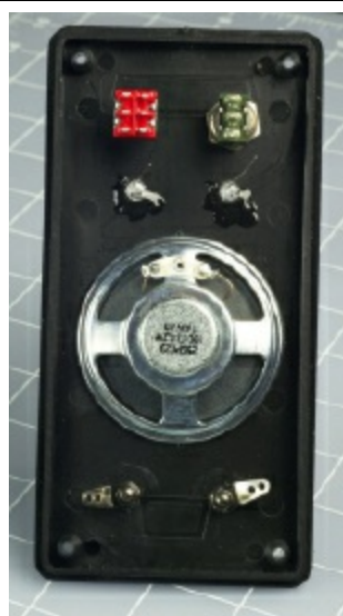
Figure 3-109. Components have been added to the control panel of the project box (seen from the underside). The budspeaker has been glued in place. Spare glue was dabbed onto the LEDs, just in case. The SPDT on/off switch is at the top right, the DPDT pushbutton is at top left, and the binding posts, which will connect with the network of magnetic sensor switches, are at the bottom.
