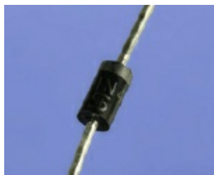
Figure 3-30. This 1N4001 diode is about 1/4 inch long and can handle up to 50 volts.
