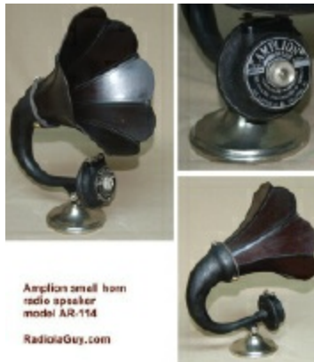
Figure 5-28. This beautiful Amplion AR-114x illustrates the efforts of early designers to maximize efficiency in an era when the power of audio amplifiers was very limited. Photos by "Sonny, the RadiolaGuy." Many early speakers are illustrated at www.radiolaguy.com . Some are for sale.
