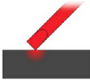
Figure 3-45. With only a small surface area of contact between the iron and the working surface, an insufficient amount of heat is transferred.
