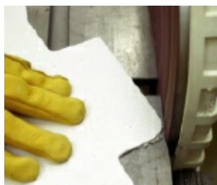
Figure 5-82. A belt sander or disc sander is the ideal tool for rounding corners when working with ABS plastic.
