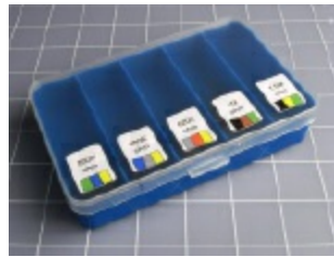
Figure 5-6. To check that resistors are not placed in the wrong compartments, print the color code on each label.
