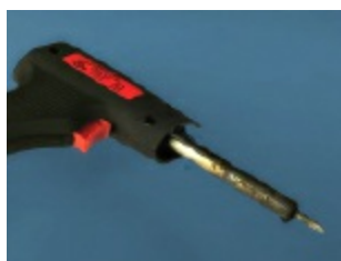
Figure 3-2. This higher-wattage soldering iron delivers the additional heat necessary for thicker wire or larger components.
