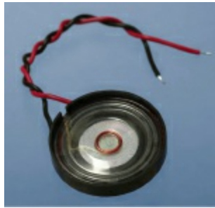
Figure 2-16. This miniature budspeaker, just over 1 inch in diameter, is useful for verifying audio output direct from transistor circuits.
