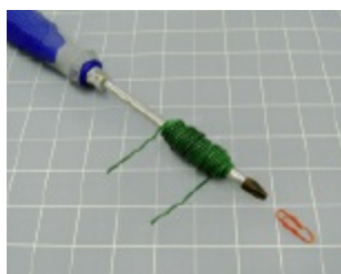
Figure 5-11. Anyone who somehow missed this most basic childhood demo of electromagnetism should try it just for the fun of proving that a single AA battery can move a paper clip.
