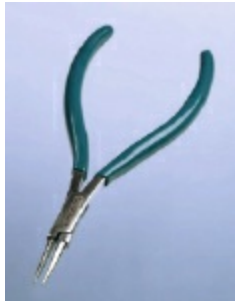
Figure 1-3. Sharp-pointed pliers are designed for making jewelry, but are also useful for grabbing tiny components.
