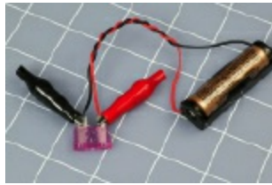
Figure 1-35. When you attach both wires to the fuse, the little S-shaped element inside will melt almost instantly.
