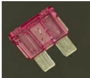
Figure 1-37. The same fuse after being melted by electric current.
