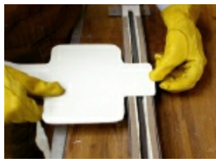
Figure 5-85. Making clean, precise bends in ABS is simply a matter of resting the plastic over a bender that consists of an electric heating element.
