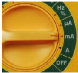
Figure 1-58. Any meter will blow its internal fuse if you try to make it measure too high an amperage. In our circuit, this is not a risk as long as you keep the potentiometer in the middle of its range. Choose “mA” for milliamps and remember that the meter displays numbers that mean thousandths of an amp.
