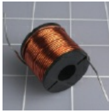
Figure 5-46. The black tape is removed, revealing a coil of magnet wire.
