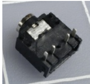
Figure 5-126. Closeup of the 3.5-mm stereo socket that is used with the USB download cable.
