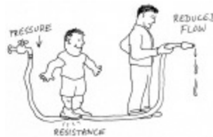
Figure 1-34. Larger resistance results in smaller flow—but if you increase the pressure, it may overcome the resistance and increase the flow.
