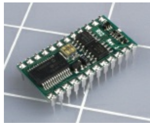
Figure 5-149. The BASIC Stamp controller consists of surface-mounted components on a platform that has pins spaced at 1/10-inch intervals, for insertion in a breadboard or perforated board. This component uses a version of BASIC that is similar to the programming language of the PICAXE, but has many more extensions. The BASIC Stamp is available for use with a wide range of peripheral devices, including many alphanumeric dot-matrix displays.
