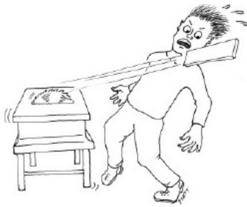
Figure 5-76. The perils of kickback. Plastic easily sticks to the blade of a table saw, which will hurl it at you unexpectedly. Use other tools to cut plastic.
