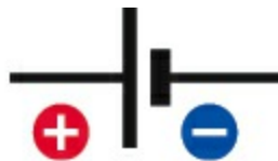
Figure 2-44. The battery symbol is usually shown without + and - symbols. I've added them for clarity.
