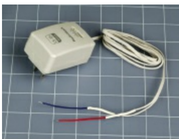
Figure 3-51. Solid-core color-coded wires, soldered onto the wires from an AC adapter, provide a convenient way to feed power to a breadboard. Note that the wires are of differing lengths to reduce the risk of them touching each other.
