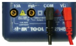
Figure 1-20. To measure resistance and voltage, plug the black lead into the Common socket and the red lead into the Volts socket. Almost all meters have a separate socket where you must plug the red lead when you measure large currents in amps, but we'll be dealing with this later.
