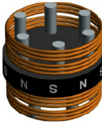
Figure 5-114. This 3D rendering gives a better idea of what a typical stepper motor looks like inside. The copper coils and gray cylinders are stationary, while the black disc rotates between them.
