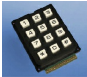
Figure 4-10. When shopping for a numeric keypad, it should have 12 keys in “touchtone phone” layout, and should have at least 13 contacts for input/output. The contacts are visible here along the front edge.
