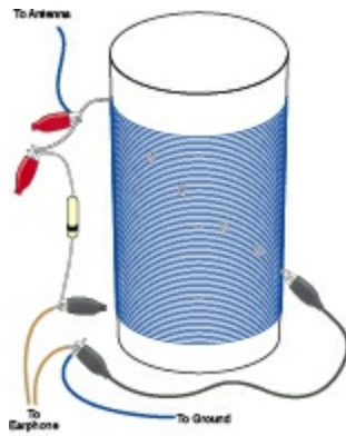
Figure 5-66. A signal from the antenna can pass through the coil to ground. If the jumper wire is attached to an appropriate tap on the coil, it resonates with the radio signal, just powerfully enough to energize the earphone which is wired in series with a diode.
