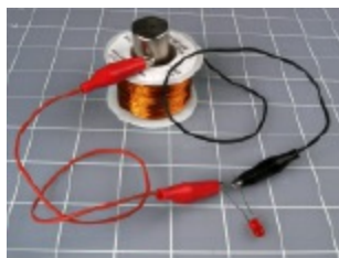
Figure 5-21. By moving a magnet vigorously up and down through the center of a coil, you generate enough power to make the LED flash brightly.
