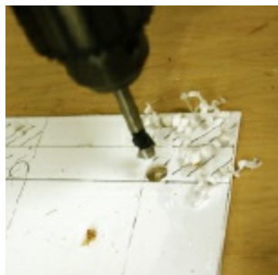
Figure 5-84. By drilling holes at any location where two bends intersect, you reduce the risk of the plastic fissuring.
