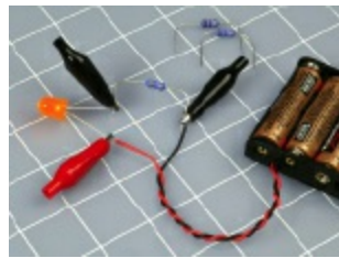
Figure 1-44. The setup for Experiment 3 , showing resistors of 470 \Omega , 1K \Omega , and 2K \Omega . Apply alligator clips where shown, to make a secure contact, and try each of the resistors one at a time at the same point in the circuit, while watching the LED.
