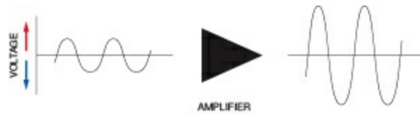
Figure 5-31. Step 3: the tiny signals from the microphone pass through an amplifier, which enlarges their amplitude while retaining their frequency and the shape of their waveform.
