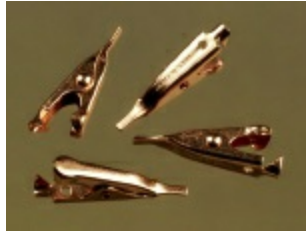
Figure 3-22. These small clips absorb heat to protect components when you're soldering them.
