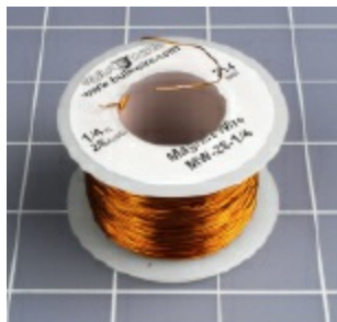
Figure 5-19. Magnet wire has thinner insulation than hookup wire, allowing the turns to be more densely packed, inducing a more powerful magnetic field.
