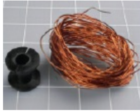
Figure 5-47. The audio crossover coil consists of a plastic spool and some wire. Nothing more.
