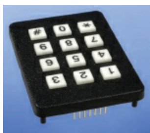
Figure 4-11. This keypad has insufficient pins and will not work in the circuit in this book.
