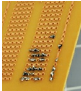
Figure 3-100. After soldering, the leads are snipped short and the joints are inspected under a magnifying glass. Another two or three components can now be inserted, and the process can be repeated.
