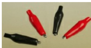
Figure 1-11. Alligator clips inside vinyl sheaths, which reduce the chance of accidental short circuits.
