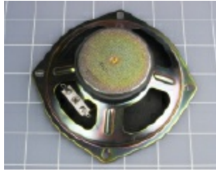
Figure 5-35. To hear the effects of audio filters using coils and capacitors, you'll need a loudspeaker capable of reproducing lower frequencies. This 5-inch model is the minimum required.
