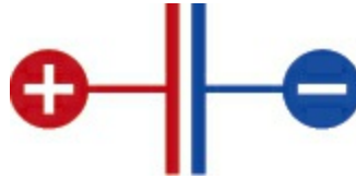
Figure 2-67. When DC voltage reaches a capacitor, no current flows, but the capacitor charges itself like a little battery. The positive and negative charges are equal and opposite.
