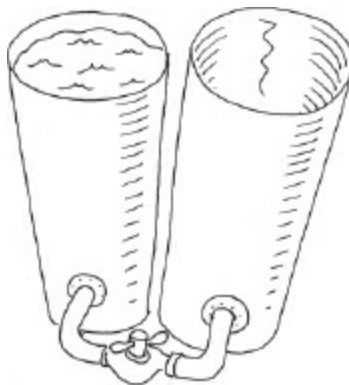
Figure 1-26. Think of the cells in a battery as being like two cylinders: one full of water, the other empty. Open a connection between the cylinders, and the water will flow until the levels are equal on both sides. The less resistance in the connection, the faster the flow will be.
