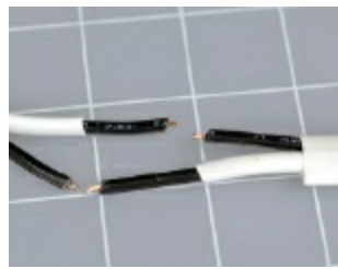
Figure 3-58. Figures 3-52 through 3-58 illustrate the sequence of steps to prepare for making a shortened power cord for a laptop computer power supply.
