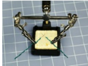
Figure 3-31. A helping hand work aid is shown here holding two wires with their stripped ends touching. The magnifying glass has been hinged out of the way.
