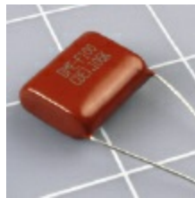
Figure 5-44. Some nonelectrolytic capacitors have no polarity, such as this high-quality polyester film capacitor. However, they tend to be much more expensive, and are hard to find in values higher than 10 \mu\text{F} .
