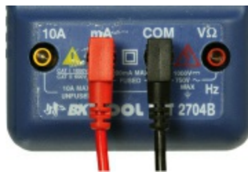
Figure 1-61. A manual meter such as the one here may require you to shift the red lead to a different socket, to measure milliamps. Most modern meters don't require this until you are measuring higher currents.
