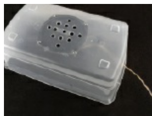
Figure 5-39. A resonant enclosure is necessary if you want to hear some bass (lower frequencies) from your speaker. A cheap plastic shoebox is sufficient for demo purposes.
