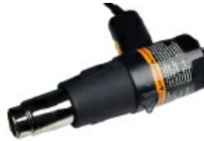
Figure 3-9. Like an overpowered hair dryer, the heat gun is used with heat-shrink tubing to create a snug, insulated sheath around bare wire.
