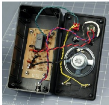
Figure 3-111. The circuit board has been installed in the base of the project box, and the power input jack has been screwed into the end of the box. Twisted wire-pairs have been connected on a point-to-point basis, without much concern over neatness, as this is a relatively small project. The white insulation at the top-right corner of the front panel is heat-shrink tube that encloses a solder joint and the 680Ω load resistor. Soldering wires to the pushbutton switch requires care and precision, as the contacts are closely spaced.
