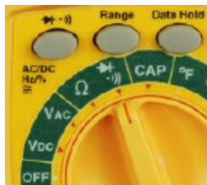
Figure 2-32. To check a circuit for continuity, turn the dial of your meter to the symbol shown. Only use this feature when there is no power in the component or the circuit that you are testing.
