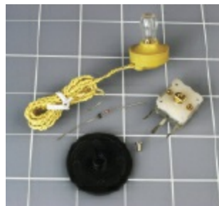
Figure 5-59. Just add wire and a coil, and this is all you need to receive AM radio signals. The black disc becomes the tuning dial, after it is screwed onto the variable capacitor (right). This is actually an optional extra. A germanium diode (center) rectifies the radio signal. The high-impedance earphone (top) creates a barely audible sound.
