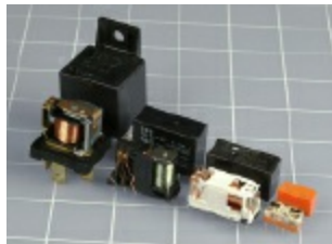
Figure 2-57. Four assorted 12-volt relays, shown with and without their packages. The automotive relay (far left) is the simplest and easiest to understand, because it is designed without much concern for the size of the package. Smaller relays are more ingeniously designed, more complex, and more difficult to figure out. Usually, but not always, a smaller relay is designed to switch less current than a larger one.
