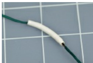
Figure 3-48. Slip the tubing over your wire joint.
