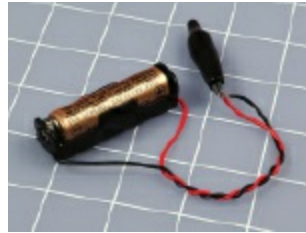
Figure 1-32. Shorting out an alkaline battery can be safe if you follow the directions precisely. Even so, the battery is liable to become too hot to touch comfortably. Don't try this with any type of rechargeable battery.
