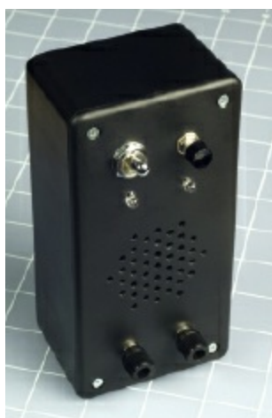
Figure 3-114. The intrusion alarm completed and in its project box.
