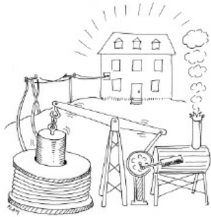
Figure 5-22. Because inductance increases with the diameter of a coil and with the square of the number of turns, your power output from moving a magnet through the coil can increase dramatically with scale. Those wishing to live "off the grid" may consider this steam-powered configuration, suitable for powering a three-bedroom home.
