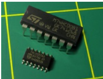
Figure 4-3. The DIP chip, at the rear, has pins spaced 1/10 inch apart, suitable for insertion in a breadboard or perforated board. It can be soldered without special tools. The small-outline integrated circuit (SOIC) surface-mount chip (foreground) has solder tabs spaced at 1/20 inch. Other surface-mount chips have pins spaced at 1/40 inch or even less (these dimensions are often expressed in millimeters). Surface-mount chips are designed primarily for automated assembly and are difficult to work with manually. In this photo, the yellow lines are 1 inch apart to give you an idea of the scale.
