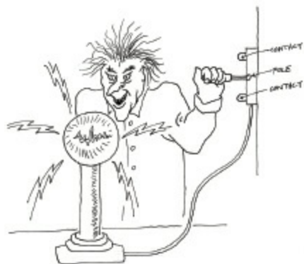
Figure 2-29. This evil mad scientist is ready to apply power to his experiment. For this purpose, he is using a single-pole, double-throw knife switch, conveniently mounted on the wall of his basement laboratory.
