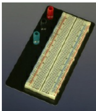
Figure 2-2. This "breadboard" for quickly constructing electronic circuits has a metal base, and screw terminals for attaching wires from a power supply.
