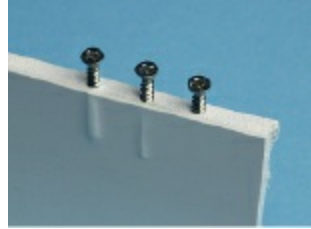
Figure 5-90. Three #4 screws driven into the edge of ABS, using a 1/16 -inch guide hole, a 5/64 -inch guide hole, and a 3/32 -inch guide hole. respectively Because the first two guides holes were too small, the plastic swelled around the screw (but did not break).
