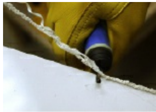
Figure 5-81. A deburring tool will clean and bevel the sawn edge of a piece of plastic in just a couple of quick strokes.
