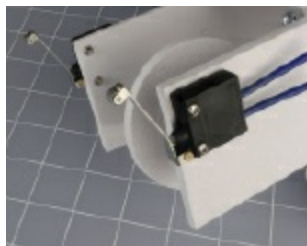
Figure 5-97. Two microswitches with metal arms are mounted on each side of the cart, where they will sense any
