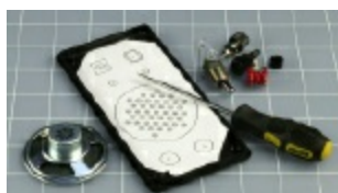
Figure 3-107. A printed layout for the switches, LEDs, and other components has been taped to the underside of the lid of the project box. An awl is pressed through the paper to mark the center of each hole to be drilled in the lid.
