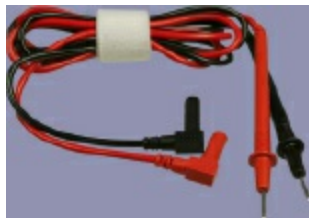
Figure 1-17. The black lead plugs into the Common (COM) socket, and the red lead plugs into the red socket that’s almost always on the righthand side of a multimeter.
