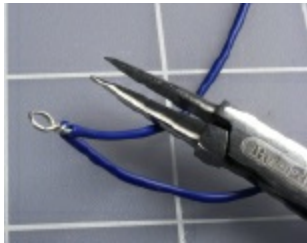
Figure 5-62. Each exposed section of wire is twisted into a loop using sharp-nosed pliers.
