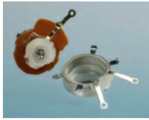
Figure 1-48. To open the potentiometer, first pry up the four little metal tabs around the edge (you can see one sticking out at the left and another one sticking out at the right in Figure 1-47). Inside is a coil of wire around a flat plastic band, and a pair of springy contacts (the wiper), which conduct electricity to or from any point in the coil when you turn the shaft.
