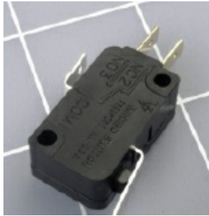
Figure 5-74. A microswitch has a small button (at the front, righthand side in this picture) that is often actuated by a pivoted metal lever. The switch can respond to a very light pressure, but can handle relatively high currents.
