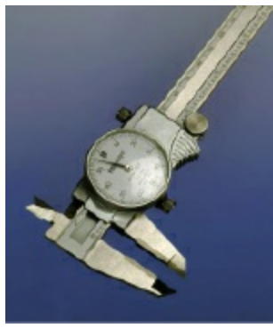
Figure 3-19. Calipers can be digital (which automatically convert from millimeters to 1/64 inch to 1/1,000 inch), or analog like these (so you never need to worry about a dead battery).
