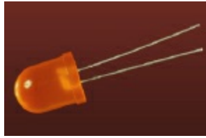
Figure 1-15. Jumbo-sized LED (1 cm diameter) is not necessarily brighter or more expensive. For most of the experiments in this book, buy whatever LEDs you like the look of.
