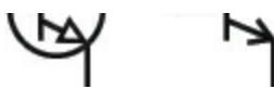
Figure 2-91. The symbol for an NPN transistor always has an arrow pointing from its base to its emitter. Some people include a circle around the transistor; others don't bother. The style of the arrow may vary. But the meaning is always the same. The top-left version is the one I use in this book.
