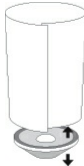
Figure 2-106. A loudspeaker emits sound from its bottom surface as well as its top surface. To increase the perceived audio volume, use a cardboard tube to separate the two sound sources, or mount the speaker in a small box.
