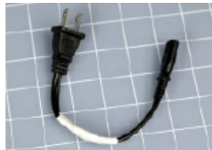
Figure 3-65. Completion of the shortened power cord for a laptop power supply.
