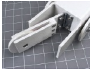
Figure 5-95. A closeup of the hinged trailing wheel, which rotates freely and can flip from side to side with minimal friction.
