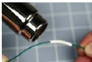
Figure 3-49. Apply heat to the tubing.
