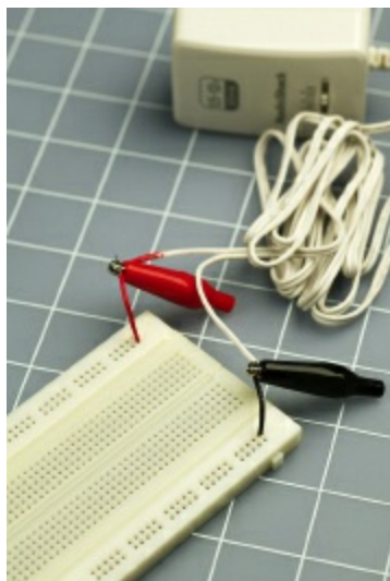
Figure 2-75. If your breadboard doesn't have screw terminals, insert two short pieces of solid-core wire with stripped ends and then attach the stranded wires from the adapter using alligator clips.
