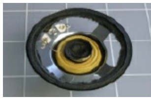
Figure 5-26. The cone has been removed.
