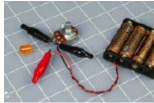
Figure 1-51. The LED in this photo is dark because I turned the potentiometer up just a little bit too far.
