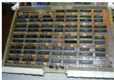
Figure 4-65. Hobbyist Bill Buzbee built himself a web server entirely from 7400 series logic chips, the oldest of which was fabricated back in 1969. The web server can be found online at http://magic-1.org , displaying pictures of itself
