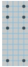
Figure 2-61. The layout of the pins of the relay, superimposed on a grid of 1/10-inch squares. This is the type of relay that you will need in Experiment 8 .
