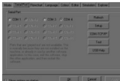
Figure 5-128. Another screenshot of the options window shows the second essential choice that you must make: selection of the COM port that the installer chose on your computer.
