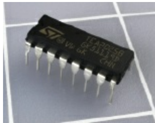
Figure 5-36. This single chip contains a stereo amplifier capable of delivering a total of 5 watts into an 8\Omega speaker when the two channels are combined.
