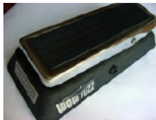
Figure 5-53. This Vox Wow-Fuzz pedal was one of the early stomp boxes, which deliberately induced the kind of distortion that audio engineers had been trying to get rid of for decades.
