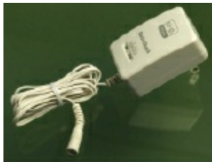
Figure 2-1. AC adapters of this general type can supply a variety of voltages, with a range as wide as 3 to 12 volts.
