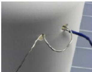
Figure 5-63. The stripped end of the wire is secured through the holes drilled in the bottle.
