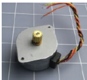
Figure 5-105. A typical stepper motor. The shaft rotates in steps when negative pulses are applied to four of the wires in sequence, the fifth wire being common-positive.
