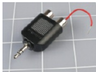
Figure 5-42. To sample the output from the headphone socket of a music player, you can use this adapter and push the stripped end of a piece of hookup wire into one of the sockets. Then use alligator clips on a jumper wire to connect the audio to your breadboarded circuit. Don't forget to use an additional jumper wire to connect the outside of the socket to the negative side of the power supply on the breadboard. Because we're only using one speaker, the amplifier is connected to only one of the stereo outputs from your player. The other is ignored.
