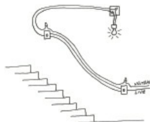
Figure 2-36. The two-switch circuit shown in Figures 2-17 and 2-35 is often found in house wiring, especially where switches are located at the top and bottom of a flight of stairs. This sketch shows what you might find inside the walls. Wires are joined with “wire nuts” inside boxes that are hidden from everyday view.
