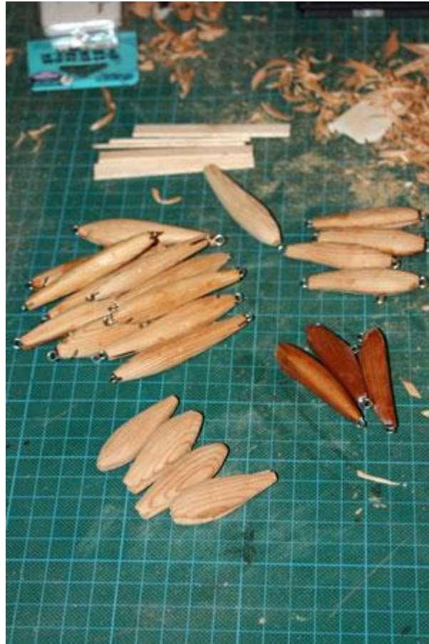
Batches of small wooden stick and jerk baits at various stages of completion.
