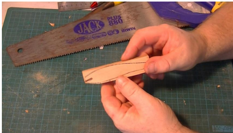
Cutting the diving lipslot, through wires slot and side profile of a medium sized crankbait.
