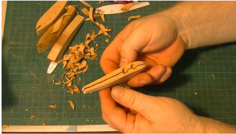
Underside of blank after removing waste from sides, top and bottom. Note the through wire slot and holes for weights.
