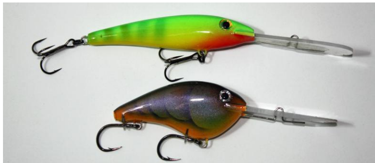
Two lures with same diving lip size, shape and angle, same tow point location and same weighting. The top one dives 3 ft (1m) deeper, due entirely to body shape.
