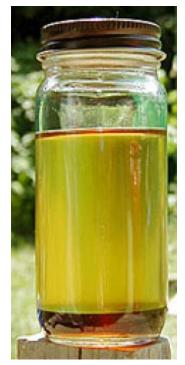
drain off the water from the bottom of the bottle by removing the duct tape from the hole. Block it again with your finger when it reaches the biodiesel. Transfer the biodiesel to the second wash bottle, add fresh water and wash again. Clean the first bottle and replace the duct tape. Repeat until finished.
