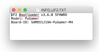
If the bootloader version you see is older than v3.9.0, you need to update. For instance, the bootloader above needs to be upgraded.
