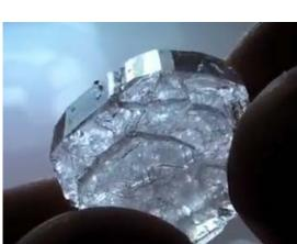
Figure 3. Piezoelectric Rochelle salt crystal made in the lab.
