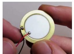
Figure 2. Ceramic Piezoelectric Transducer.
