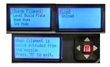
The Makerbot will turn a small motor in the extruder head. Gently feed a small piece of filament sticking out of the clear guide tube into the hole at the top of the extruder head, until the motor catches and begins pulling it down. If the motor
