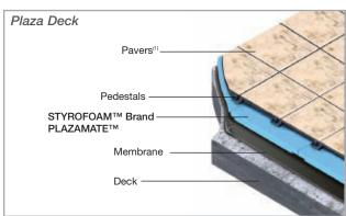
STYROFOAM™ Brand PLAZAMATE™ Insulation is designed to hold up under the heavy demands of plaza roof construction.
