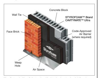
Manufactured with a distinct carbon black technology to absorb infrared radiation, STYROFOAM™ Brand CAVITYMATE™ Ultra Insulation has an R-value of 5.6 per inch. This is the highest R-value of all STYROFOAM™ Brand XPS Foam Insulation products.
