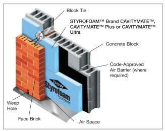
STYROFOAM™ Brand CAVITYMATE™ Insulation is designed specifically for moist cavity wall environments.
