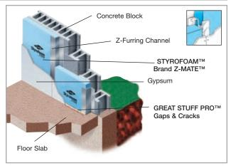
STYROFOAM™ Brand Z-MATE™ Insulation, nominally 24" wide, is pre-cut to 23-7/8", so it can be installed between Z-furring channels placed on 24" centers.
