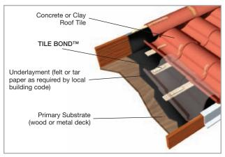
TILE BOND™ Roof Tile Adhesive adheres concrete or clay tiles to the roof deck/substrate. Refer to tile manufacturer's instructions for details.
