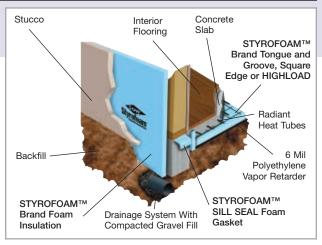
STYROFOAM™ Brand Extruded Polystyrene Foam Insulation offers excellent moisture resistance and insulating power in slab-on-grade radiant floor applications.
