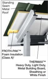
Use Class A rated THERMAX™ products in open frame designs, where the insulation boards may be left exposed to the interior. Tape top side of seams with WEATHERMATE™ Straight Flashing.
