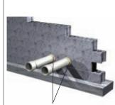
Seal smaller areas, such as gaps around pipe penetrations, with GREAT STUFF PRO™ Gaps & Cracks Insulating Foam Sealant.
