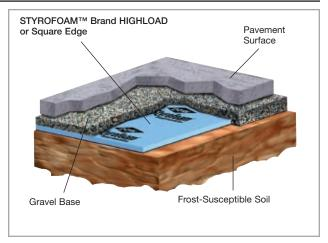
STYROFOAM  $^{\text{TM}}$  Brand HIGHLOAD Insulation has been developed specifically for in-ground applications.
