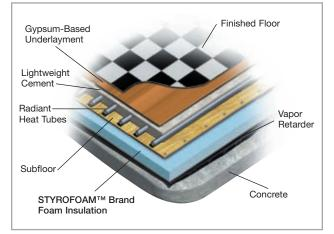
Assembly for new construction for an upper level floor or as a retrofit over existing slab. If no vapor retarder was installed under the existing slab, it is recommended to add one between the slab and the rigid foam insulation. A vapor retarder is not needed if the deck is a second-floor application.
