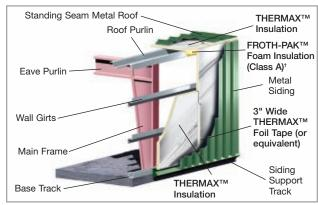
THERMAX™ Insulation products help safeguard pre-engineered metal buildings against thermal loss and moisture buildup. A variety of thicknesses and lengths up to 30' are available to meet specific design requirements.
