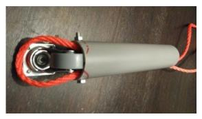
Now pull the ropes through both PVC pipes.
