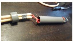
Put the endcap on the upperarm-tube. Do not glue them together. Keep them loose so that it can turn tot he left/right later, like a elbow joint.
