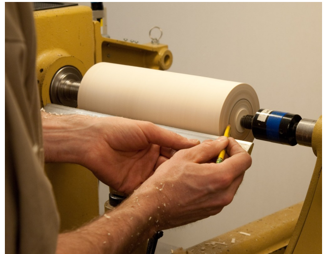
Photo 2. While the cylinder is spinning between centers, use a pencil to scribe a circle approximately 1/2 the radius. Repeat on both ends.
