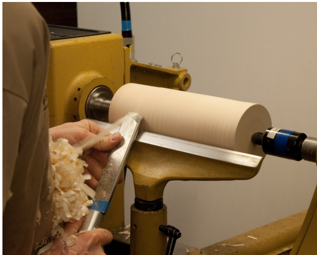
Photo 1. Mount the blank between centers (axis A), using a multi-spur drive. Using a SRG or thick cross-section skew, rough the blank into a cylinder and true up the ends.
