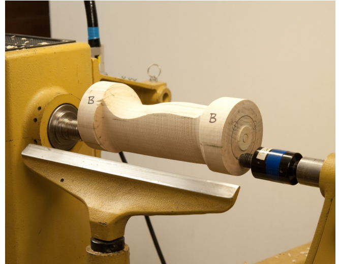
Photo 7. Observe how each ridge changes as the curved facets evolve. Remember to sneak up on each curve; stop the lathe frequently to observe the results. Creating two facets with similar curves will result in a very subtle curvature in the intersecting ridge; play with combinations of curves to see which effect appeals most to you.
