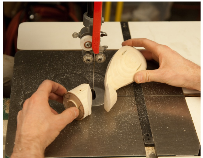
Photo 12. Use a bandsaw or other method to remove the waste wood and continue the curve of each facet to a tip. Remember to follow all safety guidelines and stay alert.
