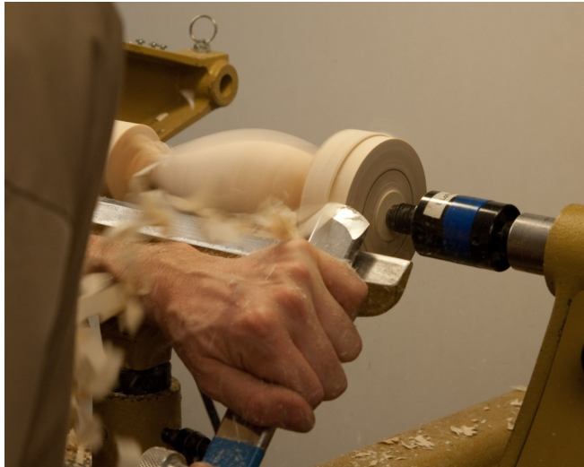
Photo 10. When you are happy with the form and quality of each facet, mount the blank between center axis (A) to remove waste wood at either end. If you are creating a stand-alone form without a separate stand, undercut the base/foot slightly so your piece sits level.
