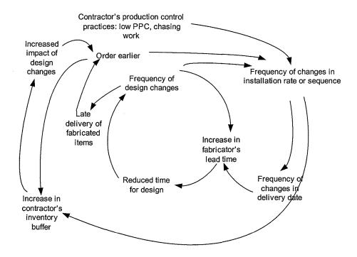
Figure 2: Interdependence of demand variability and fabrication lead
