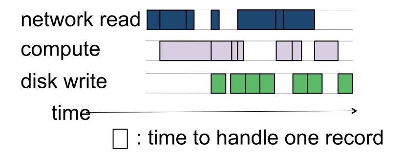
Fine-grained instrumentation needed to understand performance
