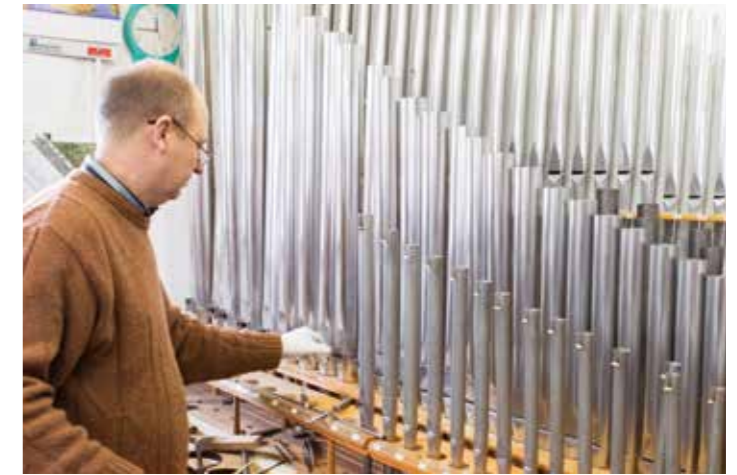
The pipes are voiced in the intonation room
