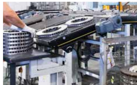
Friction rings are loaded by hand in the fully automatic aluminium foundry
