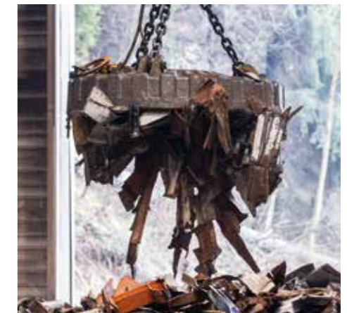
A huge magnet transports the raw materials to the production area
