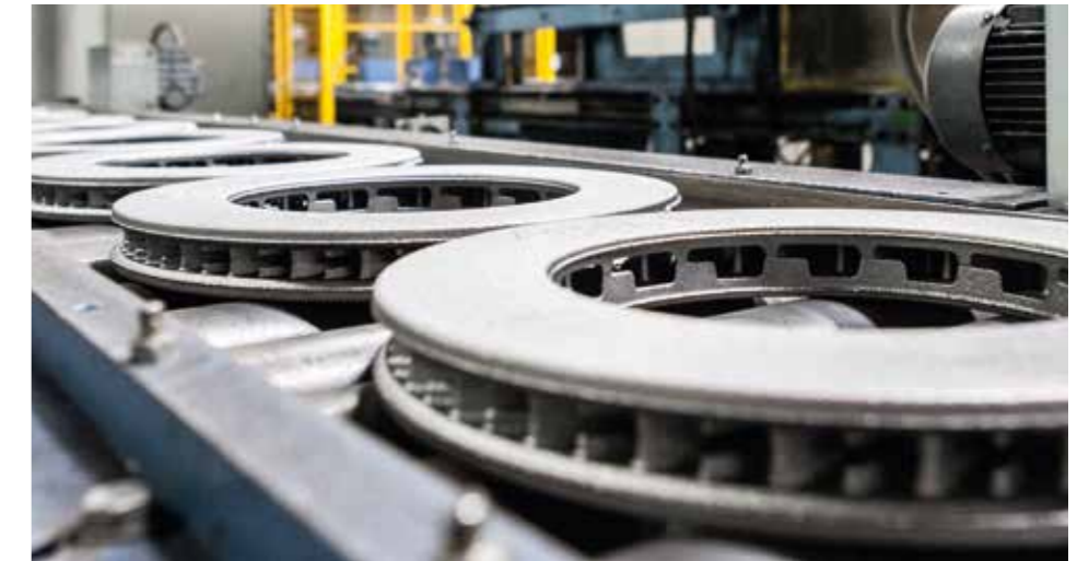
Raw friction rings roll off the production line
