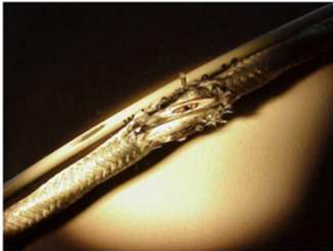
Example of a frayed fuel pump wire, representative of post-accident inspection findings on commercial aircraft (not from TWA 800)
