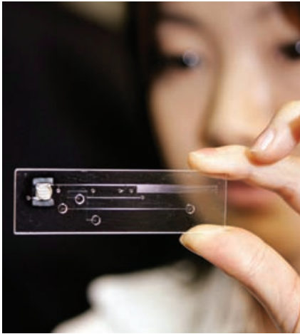
LAB ON A CHIP Launched by a Japanese company, a blood test chip using nanotechnology analyzes illness-related proteins in a drop of blood.
