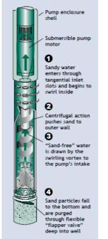
Figure 10. A cutaway diagram of a down-hole separator.
