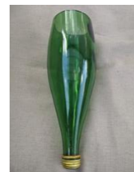
Figure 5: A glass bottle with the bottom cut off for creating a percolator
