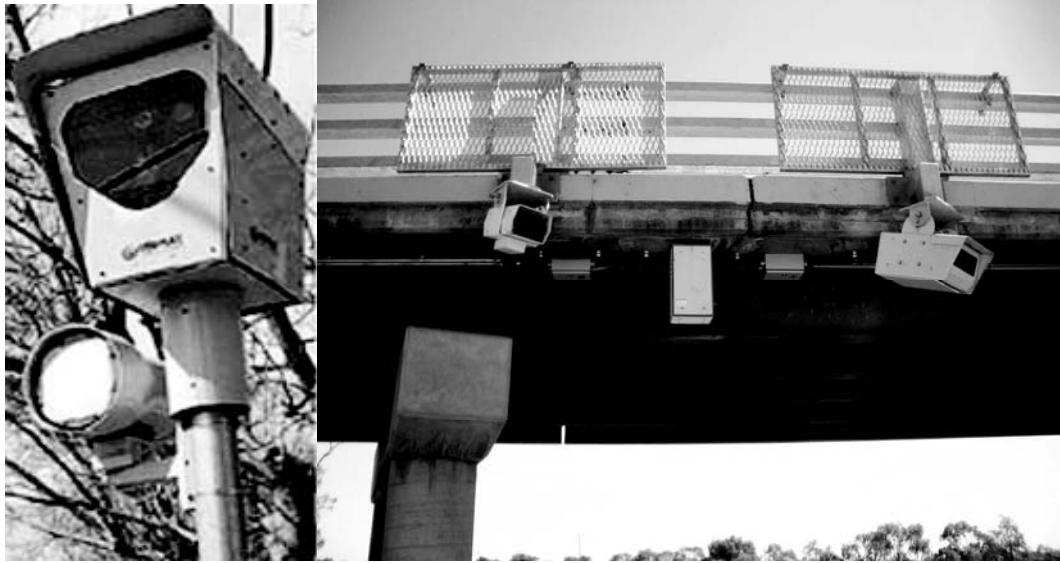
Two types of fixed camera devices used in Victoria. Left: A red-light speed fixed camera located at an intersection. Right: A speed-only fixed camera located on a highway and positioned on an overpass. (Photos courtesy of the Department of Justice.)
