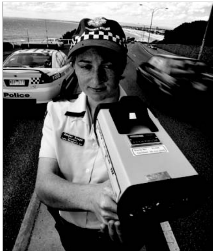
A police officer operating a hand-held laser speed detection device. (Photo courtesy of Victoria Police.)
