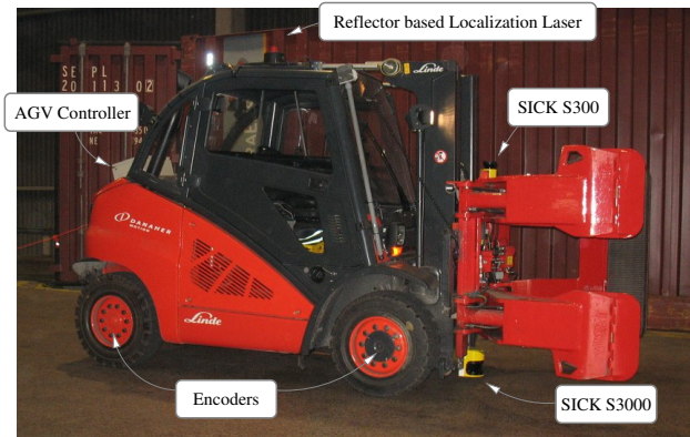
Fig. 2. The industrial truck used in the MALTA project. The truck is retrofitted with an AGV controller and a reflector-based localization laser for guidance purposes. Two SICK lasers are also added to the truck for the purposes of reel detection and safe navigation.
